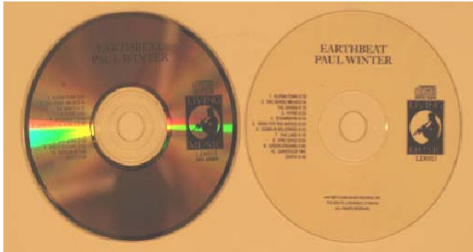
Image 4. Two CDs after 500 Hours of accelerated aging
