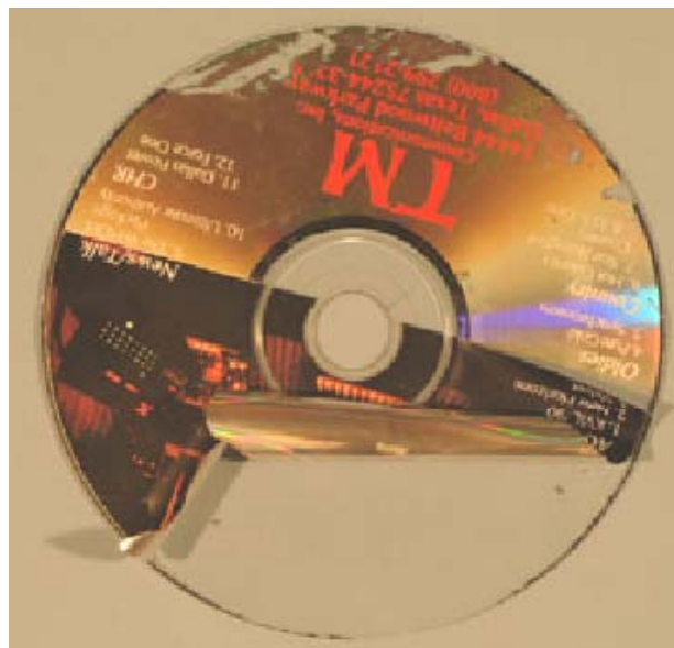
Image 5. An example of metal layer peeling and flaking from the polycarbonate substrate
